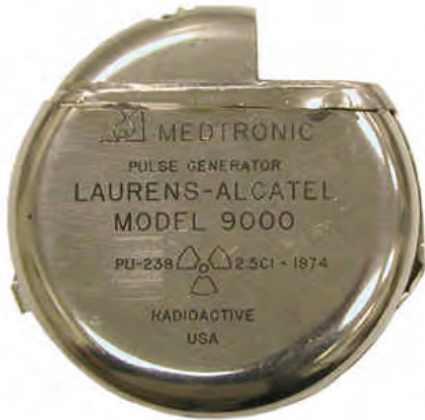
Fig. 9: The picture of the pacemaker of Medtronic company that employs 238-Plutonium radioactive source
